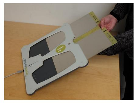
3 Insert the new electrode into the dock by gently sliding it in until the electrode is firmly aligned within the dock base.
